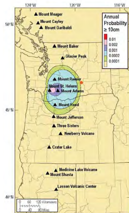
Figure 23) Probability map of at least 10.0 cm of ash accumulating as a result of a Mount St. Helen eruption.
